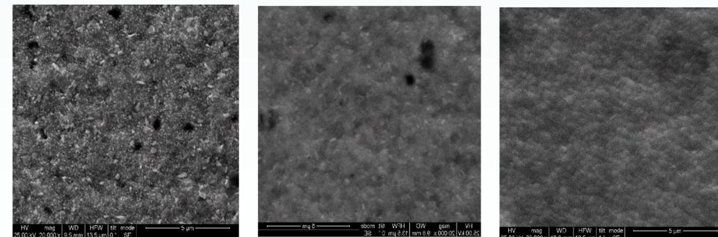
SEM images of CsCH<sub>3</sub>NH<sub>3</sub>PbI<sub>3-x</sub>Br<sub>3-x</sub> perovskite and co-sensitized perovskite-QDs PbS/CsCH<sub>3</sub>NH<sub>3</sub>PbI<sub>3-x</sub>Br<sub>3-x</sub>, CdS/CsCH<sub>3</sub>NH<sub>3</sub>PbI<sub>3-x</sub>Br<sub>3-x</sub> films.
