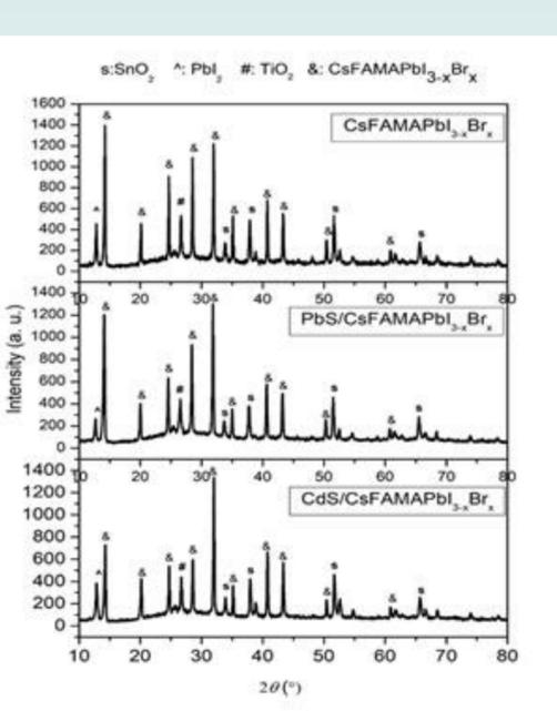
The XRPD analysis (fig. 1) confirmed the presence of the main reflections from the 3D- CsFAMAPbI<sub>3-x</sub>Br<sub>x</sub> perovskite (at 2θ = 14°, 20°). The perovskite and the co-sensitized perovskite-QDs curves are similar because the peaks of perovskite overlap those of quantum dots.
