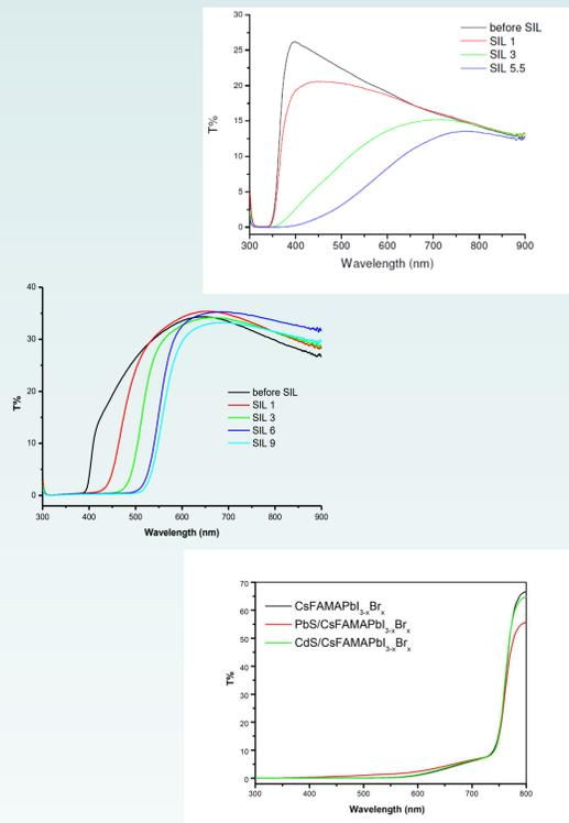
UV- Vis T% spectra of QDs , perovskite and co-sensitized perovskite-QDs films. The perovskite and the co-sensitized perovskite-QDs curves are similar, although PbS/CsFAMAPbI<sub>3-x</sub>Br<sub>x</sub> seem to have the best absorbance
